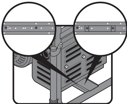
4. Assemble the rubber support on the bottom of the metal bracket and secure it with the included nut.
